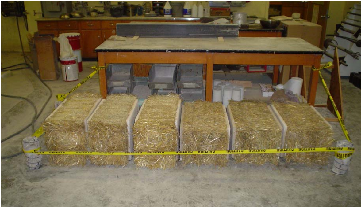
Figure 4: Completed plastered bales.
