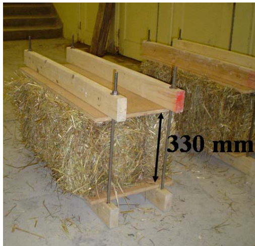
(a) Bale compressed in jig.
