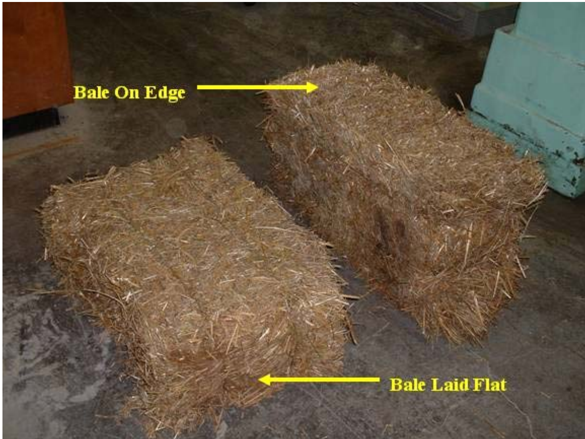
Figure 2: Bales laid flat and on edge.
